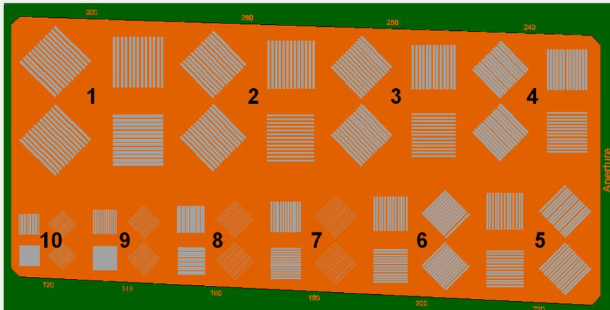
**Aperture:** The smallest pattern that can be printed without any quality problem gives the highest quantification (1- 10) for aperture result. *(the larger the better)*
