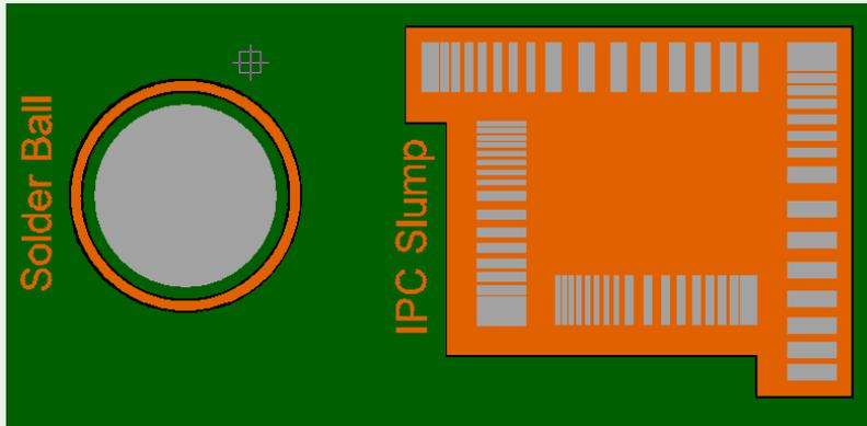
**Solder Ball:** number of satellite solderballs after reflow are counted
